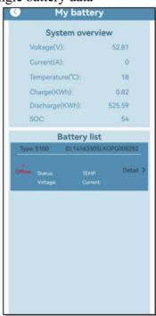
The battery overview details page displays the current battery cell data Voltage(V), Current(A), Temperature(°C), SOC, and the single cell voltage of the battery is displayed under Cell Voltage. Click Status display to view the single cell data curve
