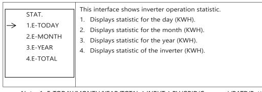
Note: 1. E-TODAY/MONTH/YEAR/TOTAL  $\rightarrow$  INPUT  $\rightarrow$  PV/GRID(Consume)/BATD(Battery discharge)  $\rightarrow$  OUTPUT  $\rightarrow$  BatC(Battery charge)/GRID(Generation)/CNSUM(Load consume)
