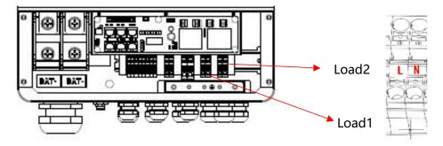
Inside the inverter, load2 is connected to load1 through a relay, and the relay disconnect when the SOC of battery is lower than set value. At this time, the load2 is powered off and load1 is still powered on. (The total power of Load1 plus Load2 should not more than the rated BACK-UP power when GRID is off)
