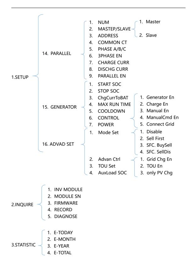
For example, Before selecting the mode, you can set it up according to the local power grid, PV input mode and battery type.
