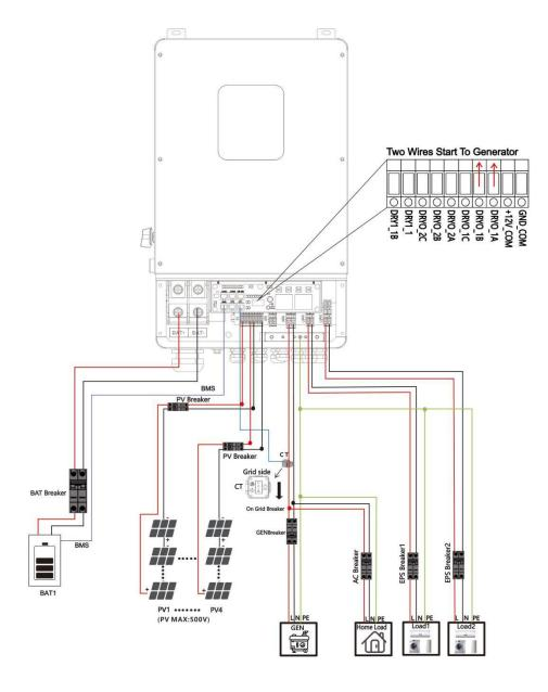
2) The Generator is normally connected to the Generator port. The connecting cable between the Generator and the inverter does not need to be covered with CT. The connection line of the power grid port should be connected
