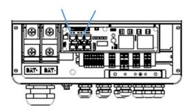
For parallel communication ,CAT 5 cables are needed. The units should be connected hand by hand.
