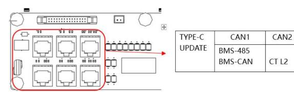
CAN1/CAN2: Communication interface for connecting inverters.
