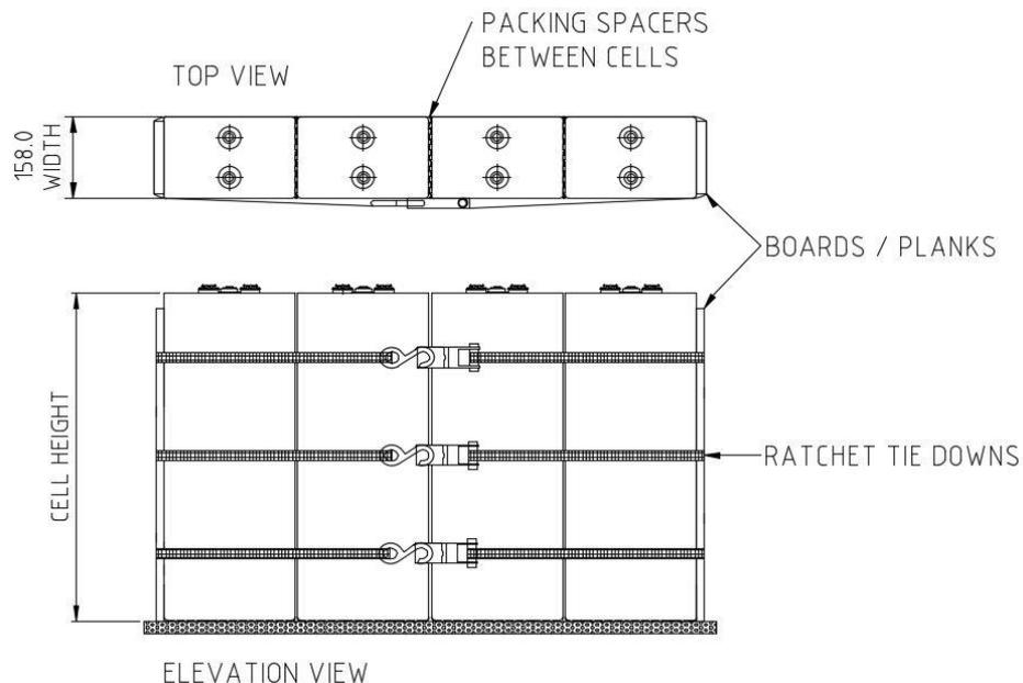
Where connectors have not yet been fitted remove the bolts, wipe the terminals clean and apply a light coating of Vaseline to the outer surface of the terminal. Connect the cells together using the inter-connectors provided ensuring that the cells are connected negative to positive throughout. When numbering the cells always begin at the positive end as cell number 1.
