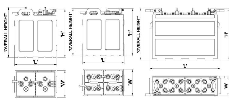
Individual cells in rugged casing to improve shock resistance and to facilitate easy cell change out if required.
