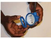
NB! Do not attempt to tighten the lens ring by any means other than the specialized tool P/N 105260 available from FNB. Failing to do so may damage the lens ring, prevent proper sealing of the lens surface to the optic gasket and render the headpiece susceptible to ingress of water and contaminants.
