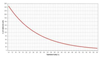
Figure 3. Typical life vs Temperature - Vented Tubular Batteries
