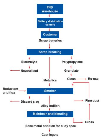
Figure 10. Typical lead recycling process
