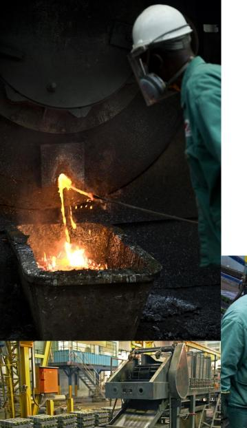
Battery plates, terminals and other extracted lead are refined and blended in the lead smelter located in Benoni to produce high quality lead alloys
