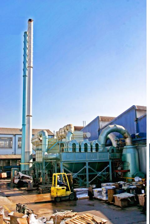
Acid is neutralised and processed through an effluent plant and properly disposed of.
