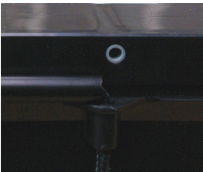
Central venting with flash arrestors
